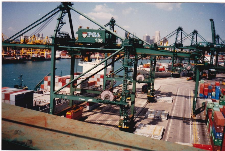
QUAY CRANE (NO.106) UNLOADING OF CONTAINER FORM A VESSEL
